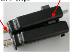
Now, bring the back edge "P" clip (USB end) of the 2<sup>nd</sup> scope down until it clicks into the 1<sup>st</sup> scope's slot. These two scopes are now mated.
